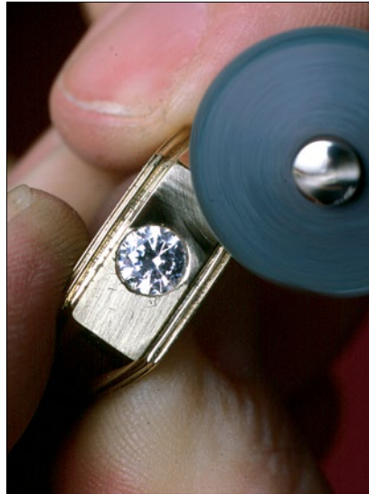
13. Use a silicone wheel to pre-polish the mounting and remove any marks.
