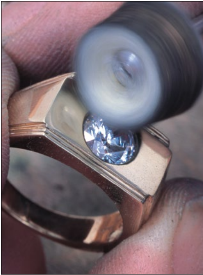
15. Use a felt buff with rouge to polish the ring, then clean thoroughly.
