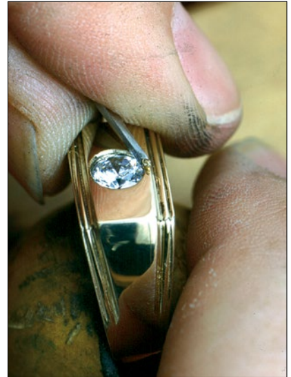
14. With a highly polished flat graver, bright cut the interior surface of the hole opening.
